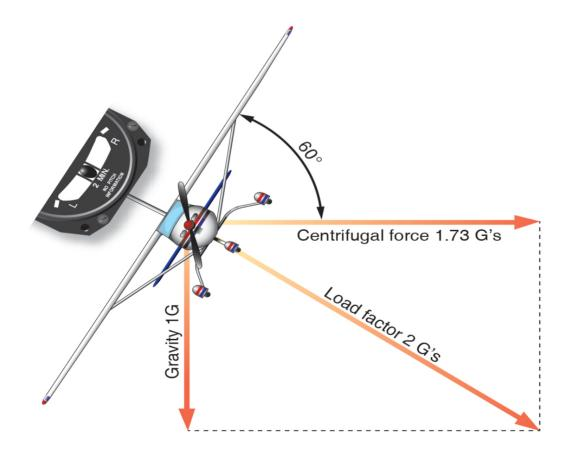
Figure 5-5. Coordinated flight in a turn.
