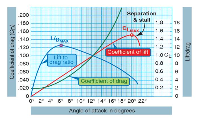
Figure 5-6. Angle-of-attack in degrees.
