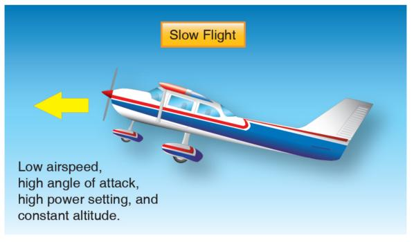
Figure 5-7. *Slow flight—low airspeed, high angle of attack, high power, and constant altitude.*
