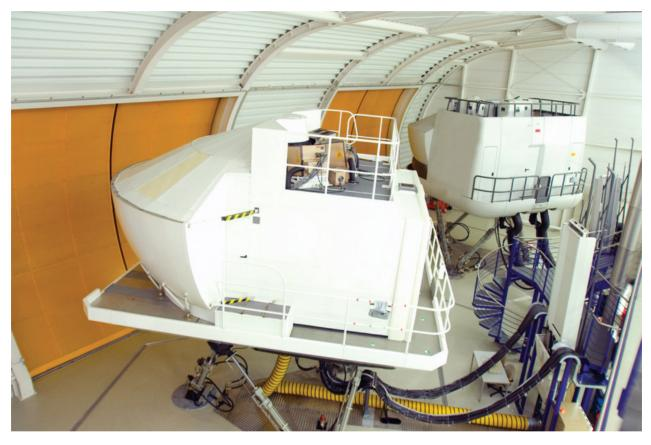
Figure 5-4. A Level D full-flight simulator could be used for UPRT.
