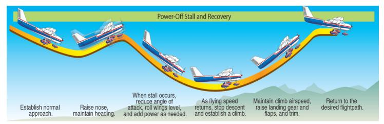
Figure 5-11. Power-off stall and recovery.
