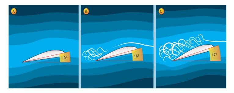
Figure 5-8. Critical angle of attack and stall.
