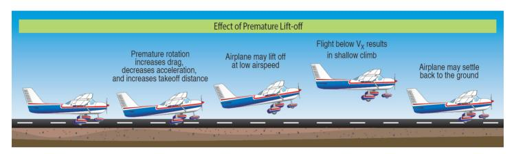
Figure 6-9. Effect of premature lift-off.
