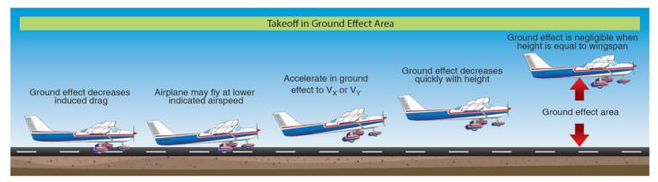
Figure 6-7. Takeoff in ground effect area.
