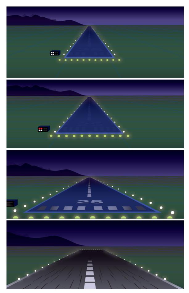
Figure 11-8. Round out when tire marks are visible.
