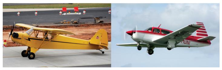
**Figure 14-1.** The Piper Super Cub on the left is a popular tailwheel airplane. The airplane on the right is a Mooney M20, which is a nose-wheel (tricycle gear) airplane.
