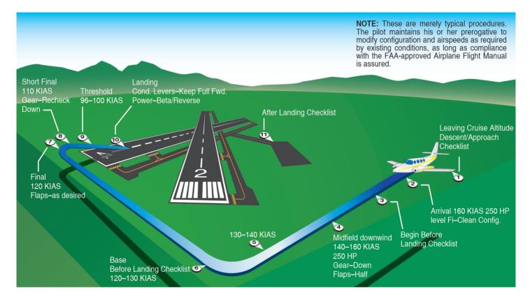
Figure 15-12. Example of a typical turboprop airplane arrival and landing profile.
