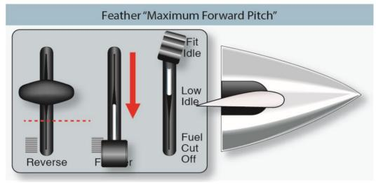
Figure 15-8C. Propeller feather (maximum forward pitch angle) characteristics.
