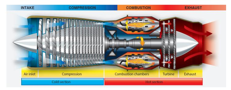
Figure 15-1. Basic components of a gas turbine engine.
