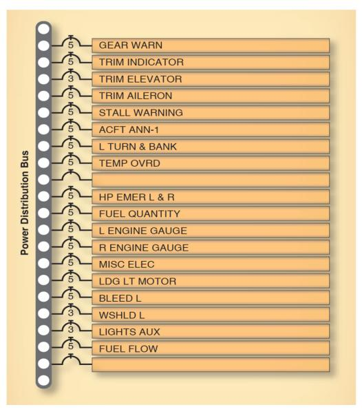
Figure 15-9. Typical individual power distribution bus.
