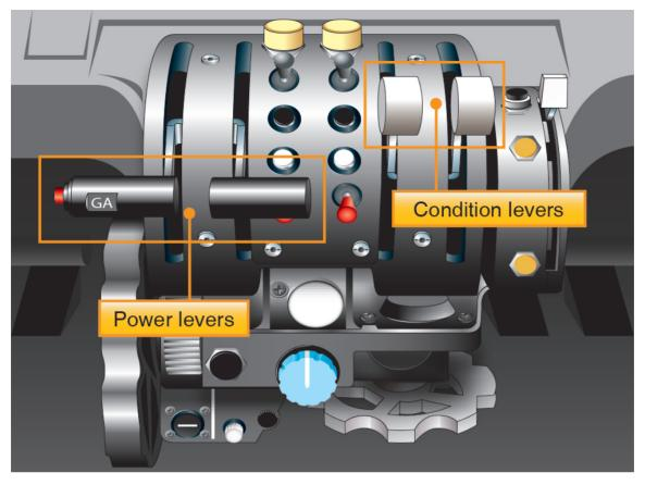
Figure 15-3. Powerplant controls—fixed-shaft turboprop engine.
