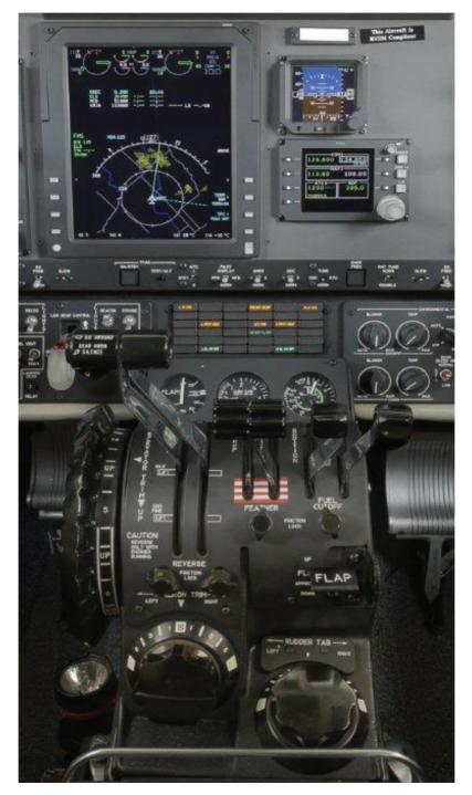
Figure 15-6. Powerplant controls—split-shaft/free turbine engine.
