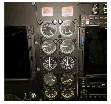
Figure 15-4. Powerplant instrumentation—fixed-shaft turboprop engine.
