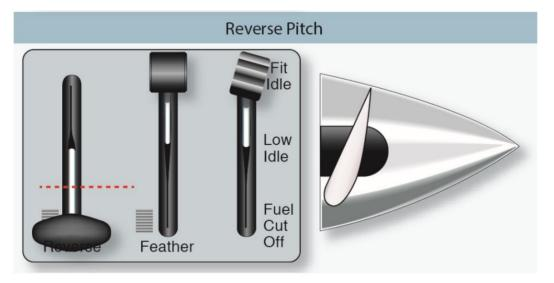
Figure 15-8D. *Propeller reverse pitch characteristics*.
