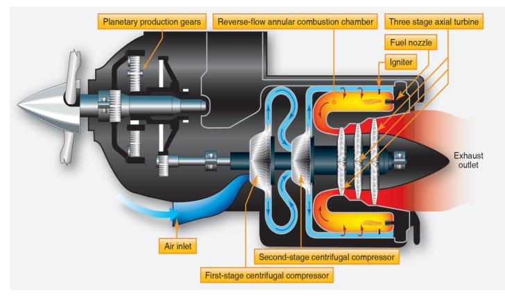
Figure 15-2. *Fixed-shaft turboprop engine*.
