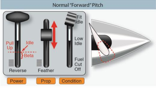
Figure 15-8A. Propeller forward pitch angle characteristics.
