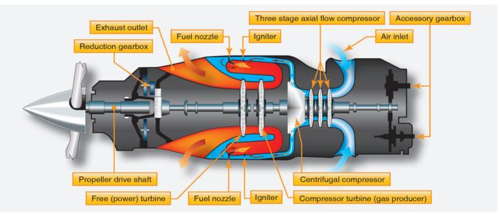
**Figure 15-5.** *Split shaft/free turbine engine.*
