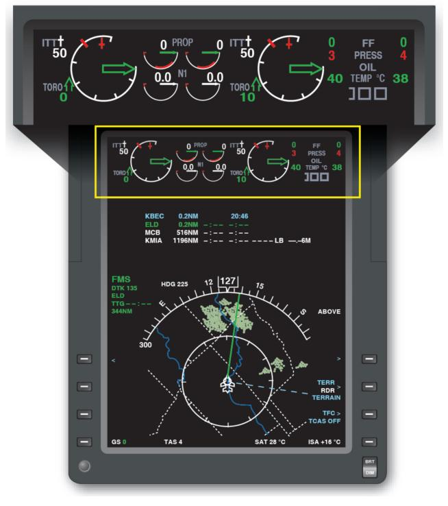
Figure 15-7. *Engine instruments—split shaft/free turbine engine.*
