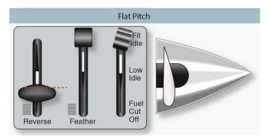
Figure 15-8B. *Propeller flat pitch characteristics*.
