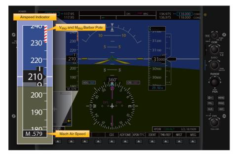
Figure 16-5. Jet airspeed indicator.
