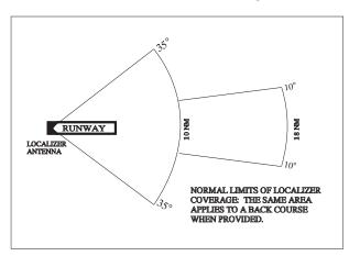
FIG 1-1-6 Limits of Localizer Coverage
