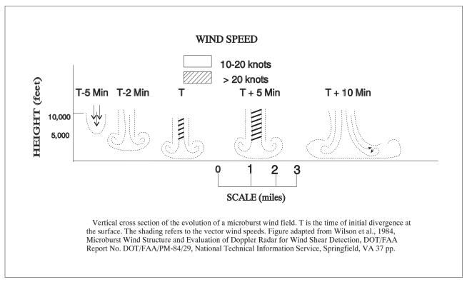
c. The life cycle of a microburst as it descends in a convective rain shaft is seen in FIG 7–1–10. An important consideration for pilots is the fact that the microburst intensifies for about 5 minutes after it strikes the ground.
