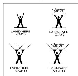
FIG 10-2-8 Recommended Landing Zone Ground Signals
