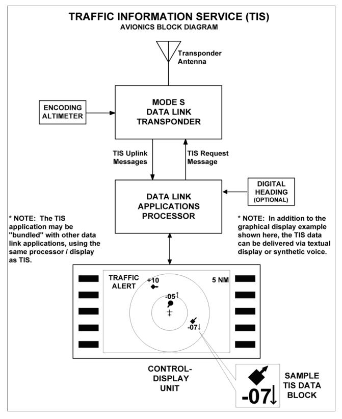
**2.** The cockpit equipment functionality required by a TIS client aircraft to receive the service consists of the following (refer to FIG 4-5-6):
