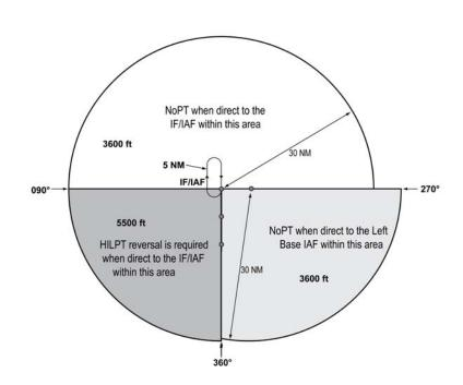
FIG 5-4-8 TAA with Right Base Eliminated
