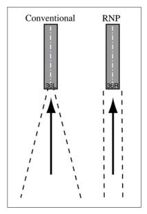
**3. RNP Parallel Approach Runway Transitions (RPAT) Operations.** RPAT approaches begin as a parallel IFR approach operation using simultaneous independent or dependent procedures. (See FIG 5–4–25). Visual separation standards are used in the final segment of the approach after the final approach fix, to permit the RPAT aircraft to transition in visual conditions along a predefined lateral and vertical path to align with the runway centerline.
