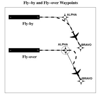
*FIG 1-2-3* Track to Fix Leg Type
