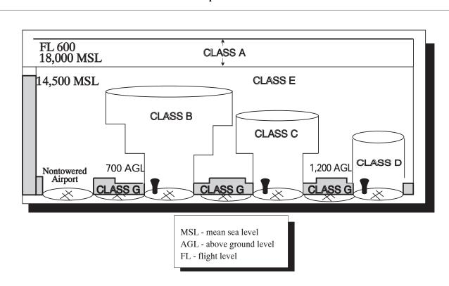
FIG 3-2-1 Airspace Classes **g. Ultralight Vehicles.** No person may operate an ultralight vehicle within Class A, Class B, Class C, or Class D airspace or within the lateral boundaries of the surface area of Class E airspace designated for an airport unless that person has prior authorization from the ATC facility having jurisdiction over that airspace. (See 14 CFR Part 103.)
