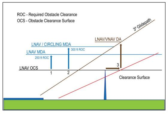
**g.** FIG 5–4–12 provides a visual representation of an obstacle evaluation and calculation of LNAV MDA, Circling MDA, LNAV/VNAV DA.
