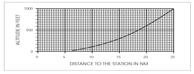
FIG 1-1-4 Service Volume Lower Edge Terminal
