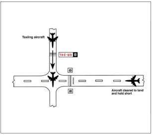
FIG 4-3-9 Land and Hold Short of a Designated Point on a Runway Other Than an Intersecting Runway or Taxiway
