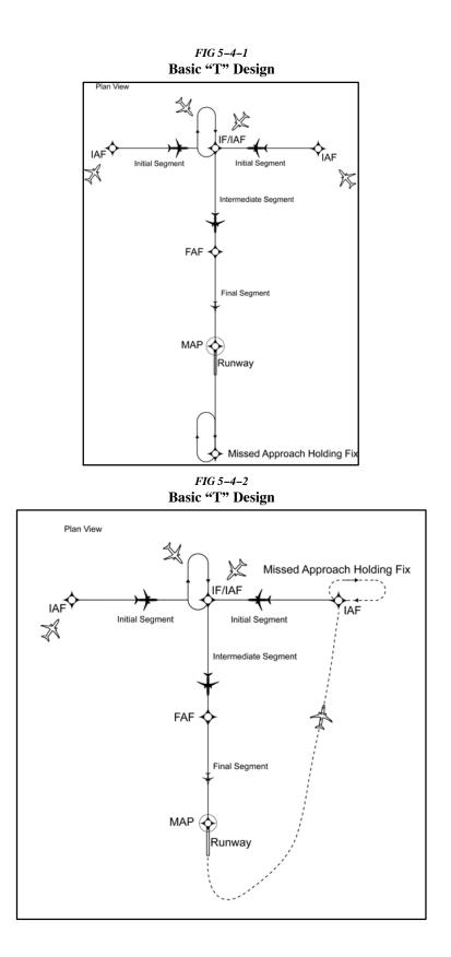
**3.** The standard TAA based on the "T" design consists of three areas defined by the Initial Approach Fix (IAF) legs and the intermediate segment course beginning at the IF/IAF. These areas are called the straight-in, left-base, and right-base areas. (See FIG 5-4-3). TAA area lateral boundaries are identified by magnetic courses TO the IF/IAF. The straight-in area can be further divided into pie-
