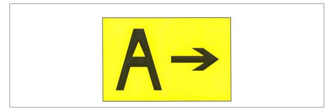
FIG 2-3-37 Direction Sign Array for Simple Intersection
