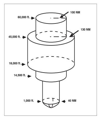
*FIG 1–1–2* **Standard Low Altitude Service Volume** (See FIG 1–1–5 for altitudes below 1,000 feet).
