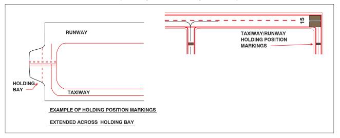
FIG 2-3-14 Runway Holding Position Markings on Runways
