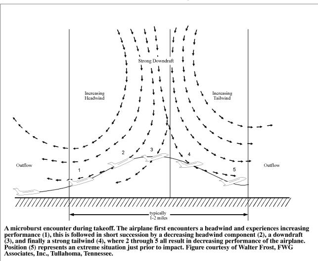
e. Microburst wind shear may create a severe hazard for aircraft within 1,000 feet of the ground, particularly during the approach to landing and landing and take-off phases. The impact of a microburst on aircraft which have the unfortunate experience of penetrating one is characterized in FIG 7–1–11. The aircraft may encounter a headwind (performance increasing) followed by a downdraft and tailwind (both performance decreasing), possibly resulting in terrain impact.
