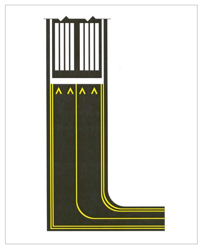
FIG 2-3-4 Displaced Threshold Markings
