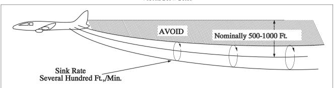
*FIG 7–3–5* Vortex Movement Near Ground – No Wind
