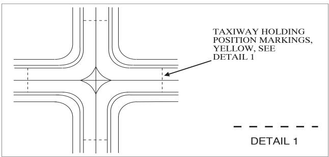
FIG 2-3-18 Vehicle Roadway Markings
