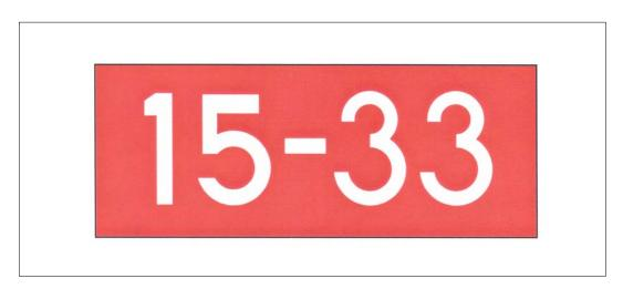
FIG 2-3-25 Holding Position Sign at Beginning of Takeoff Runway
