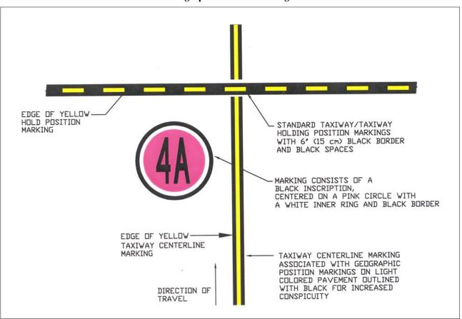
FIG 2-3-13 Runway Holding Position Markings on Taxiway
