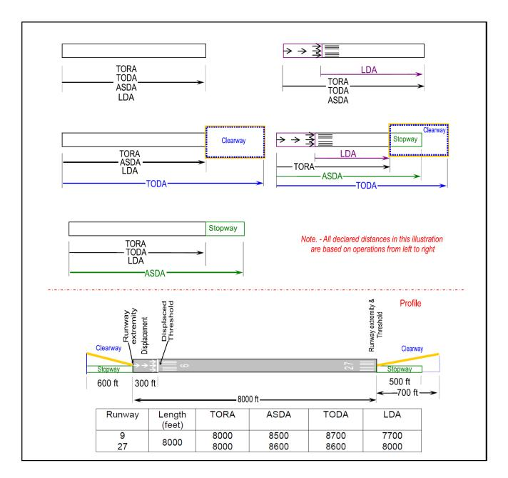
FIG 4-3-6 Effects of a Geographical Constraint on a Runway's Declared Distances
