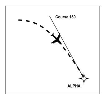
(4) **Radius to Fix.** A Radius to Fix (RF) leg is defined as a constant radius circular path around a defined turn center that terminates at a fix. See FIG 1–2–6.
