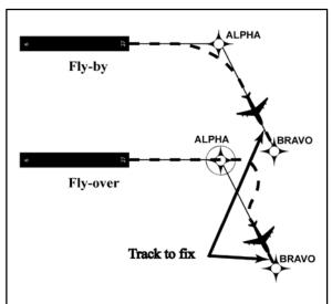
*FIG 1-2-4* Direct to Fix Leg Type
