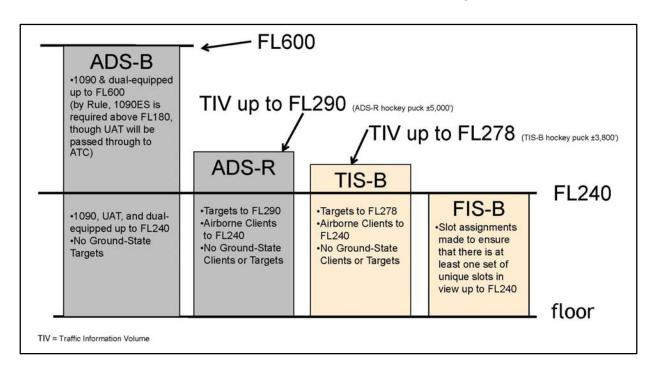
FIG 4-5-9 Terminal – ADS-B/ADS-R/TIS-B/FIS-B Service Ceilings/Floors
