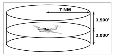
FIG 4-5-5 Terminal Mode S Radar Sites
