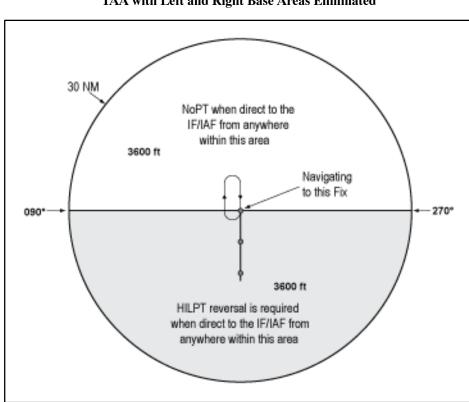
FIG 5-4-6 TAA with Left and Right Base Areas Eliminated
