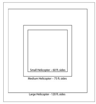
**2.** For the purposes of FIG 10–2–4 the following are provided as examples of relative helicopter size:
