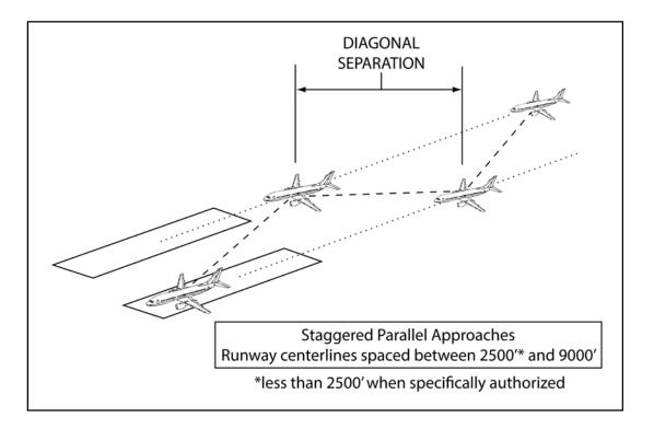
FIG 5-4-20 Simultaneous (Parallel) Dependent Approaches
