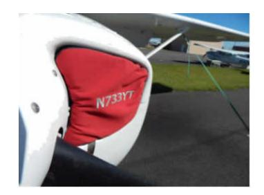
Check inside the **air intakes** for foreign matter such as bird's nests, forgotten tools, and dirt. Any found matter must be thoroughly removed before flight, as they could damage the engine or cause a fire.
