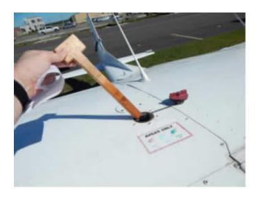
Check the diagonal **wing strut** for damage, giving emphasis to where the strut connects to the wing and the fuselage.
