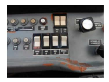
Confirm that all **circuit breakers** are in and not popped out. A popped breaker will protrude out and display two different colors, such as white and red or black and white. Notify your flight instructor if you find any popped out breakers.
