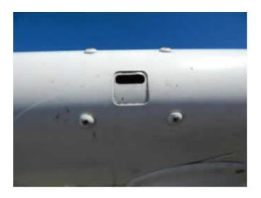
Verify that the **pitot tube** is secure. Confirm that the ram air inlet (front) and the water drain hole (bottom) are clear.
