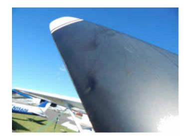
Verify that the **spinner** (nose cone) is secure and all screws are secure.
