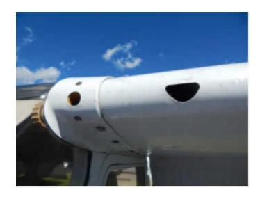
Continue down the leading edge, checking for dents and damage. Verify that the **stall** warning inlet is clear.
