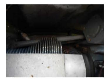
Inspect the condition of the **alternator** and **alternator belt**. Do not fly if the belt is missing, badly cracked, or excessively loose.
