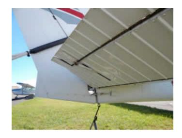
Check the elevator and **rudder cables**. Your instructor can show you these cables in more detail.
