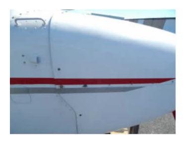
Remove the **bird plugs** from the cowling air intakes. Be careful as you do this, as the fiberglass is thin around that area and could crack if you removed them forcefully.
