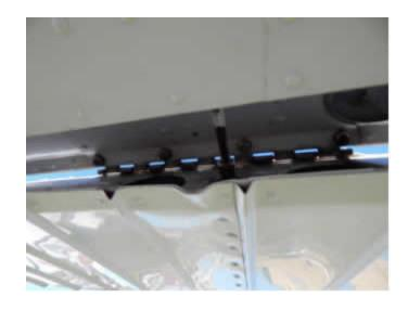
Inspect the **flap** surface above and below for damage. Push gently upwards on the flap to verify that it is being held in place. Inspect the roller bearings and tracks, and the actuator arm. Your instructor can show you these parts in more detail.
