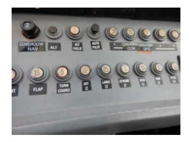
Ensure that nobody is close to the propeller, then turn the Master Switch ON. Any time the **Master Switch** is turned on, the starter could engage and possibly start the engine if certain (though rare) wiring faults existed. For this reason, is important to exercise additional caution around the propeller any time the switch is turned on.
