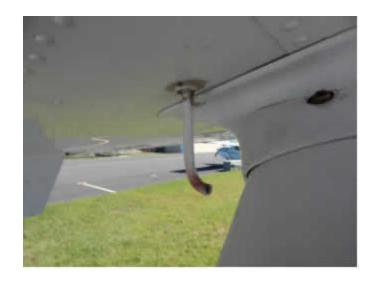
Remove the wing **tie-down** strap. If gusty wind conditions prevail, wait to remove the strap until just before you are ready to board the aircraft.
