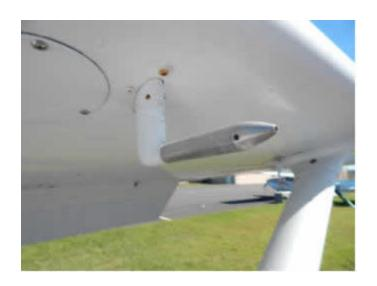
Verify that the **fuel vent** tube is secure and unobstructed
