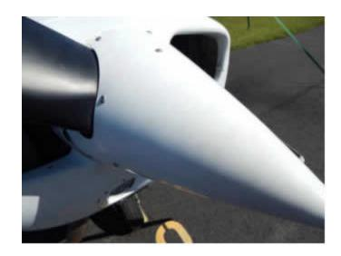
Ensure that the **carburetor air filter** is clean and unobstructed. Check for tears and clean off any foreign matter.
