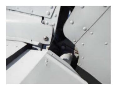
Remove the **rudder gust lock** and place it on the ground behind the aircraft. Your instructor will demonstrate the proper procedure for removing and applying the gust lock. Inspect the rudder surface and hinges. Verify that the **VOR antenna** (v-shaped) at the top of the rudder is secure.
